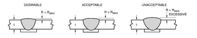
FIGURE A - WELD PROFILES FOR BUTT JOINT REQUIREMENTS (see Tables 2 and 3)
