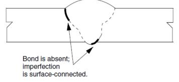
FIGURE E – Incomplete Fusion at Root of Bead or Top of Joint (IF)
