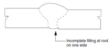
FIGURE D – Inadequate Penetration Due to High-Low (IPD)
