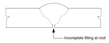
Note: One or both root faces may be inadequately filled at the inside surface. FIGURE C – Inadequate Penetration Without High-Low (IP)
